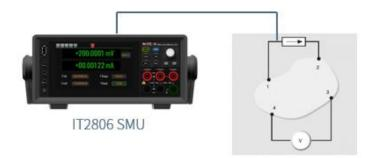
Summary: IT2800 series high-precision source/measure unit can accurately realize the resistivity test of semiconductor sheet resistance, thus providing data basis for the improvement of semiconductor manufacturing process. IT2800 SMU provides professional testing solutions for the industry due to its high-precision measurement and rich advantages of probe station fixtures.
